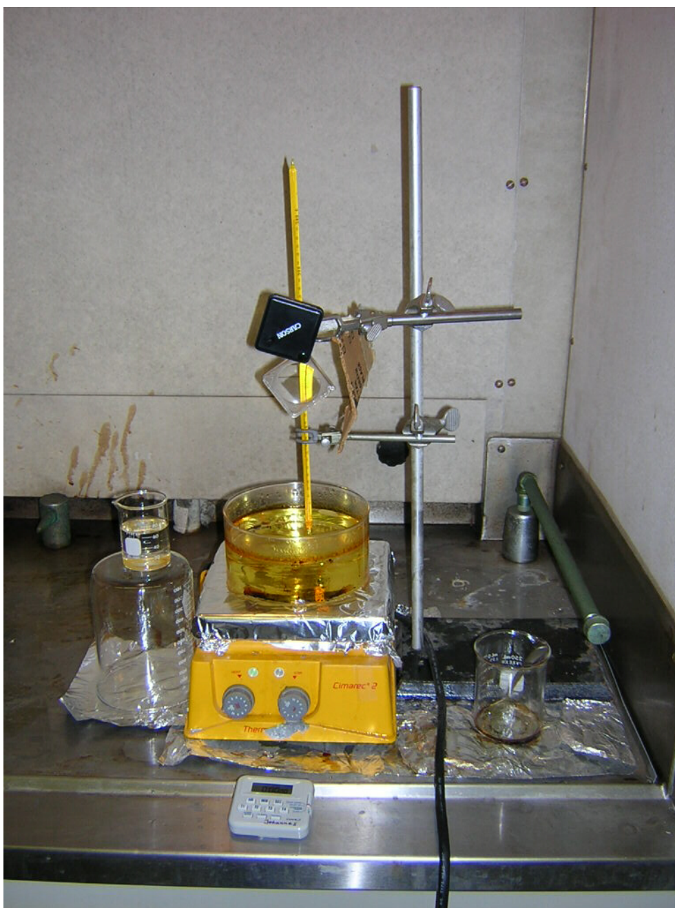
Figure 5.3: (Color). Experimental setup of the immersion experiment. Safflower oil (in a large jar on the hot plate) is used to anneal a sample on short timescales by immersion. Subsequently, the sample is immersed rapidly into ethylene glycol (liquid on the left of the hot plate in the small jar). The oil temperature is measured with a mercury thermometer. The thermometer is immersed into the oil up to the calibration line, which is indicated on the thermometer. The scale is read through a magnifying glass for higher precision. A timer is located in the front.
